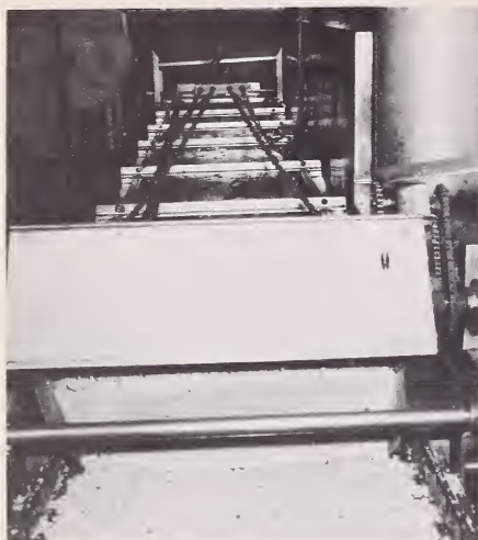
FIGURE 28.—Peanuts are oil roasted in a continuous cooker at 350 degrees F. for about 5 minutes.
